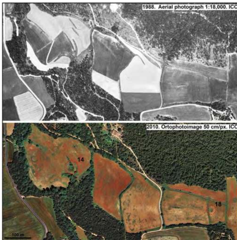
Fig. 8. Airborne images from 1988 and 2010 illustrating the geomorphic effects of the last drought period (1998–present) in the vicinity of Can Cademont within the study area. The lower image shows sinkholes 14 and 18, formed in November 1998 and in 2005–2006.
